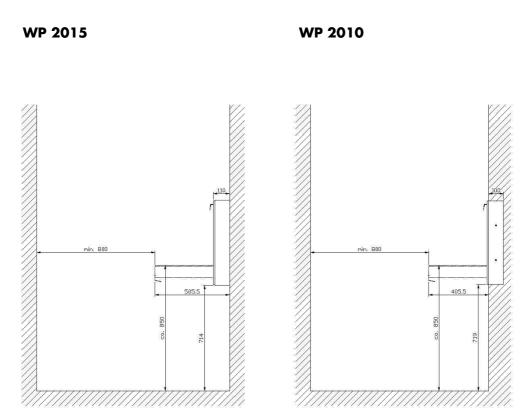
• The lateral distance to the existing wall must be sufficiently large to allow the flap to be opened and to prevent any risk of fingers, clothing, etc. becoming trapped.
